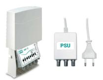
1-input (UHF) mast amplifier with 42dB gain and up to  $116dB\mu V$  output level on UHF band, gain adjustment 0-15dB and low noise figure. 694MHz 5G and 4G LTE integrated filter. Power supply included in the package.
